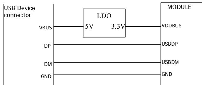
**Figure 10: USB interface circuit**
