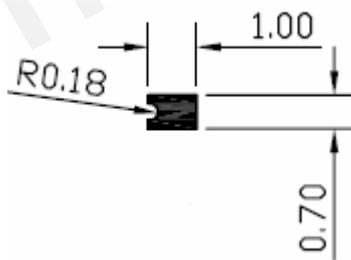
Figure 18: PAD Bottom dimensions (Unit:mm)
