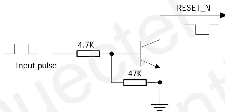
**Figure 2: Reference reset circuit using OC circuit**
