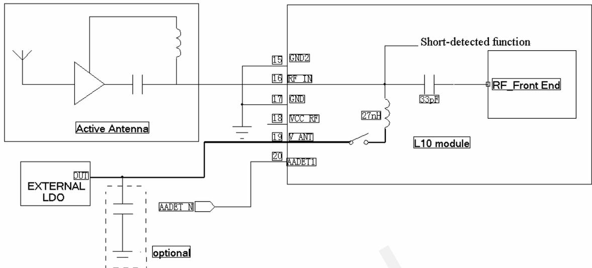
**Figure 15: Active antenna with external LDO**
