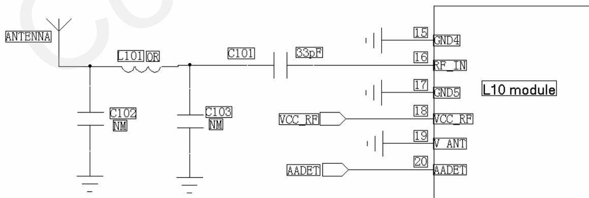
Figure 12: Reference design for passive antenna
