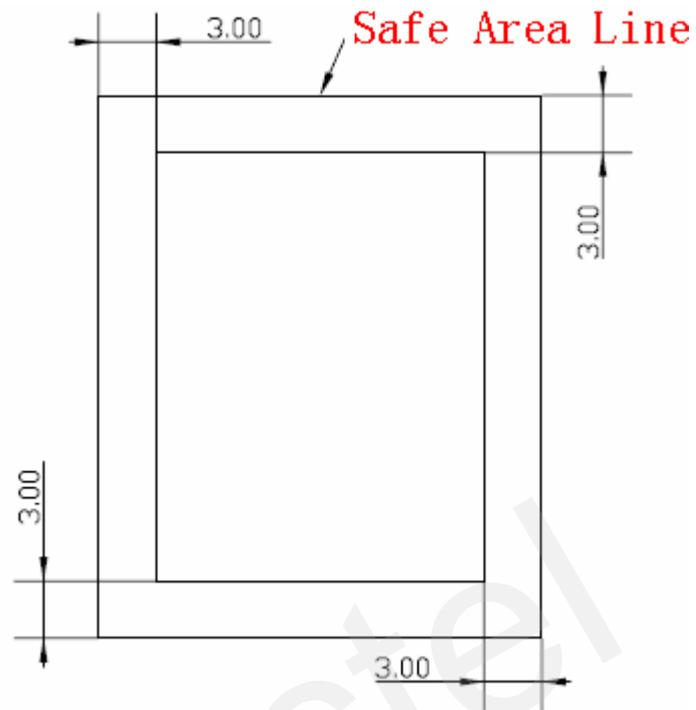
**Figure 19: Footprint of recommendation (Unit:mm)**
