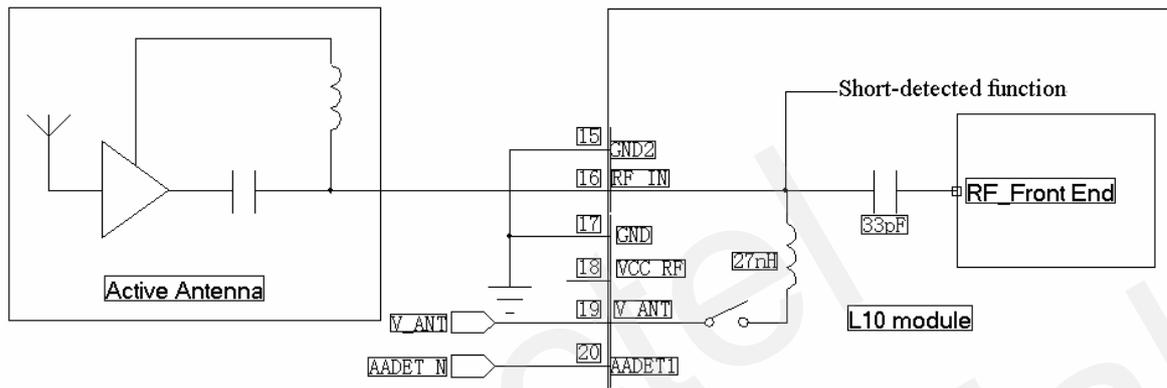
**Figure 13: Active antenna biasing**
