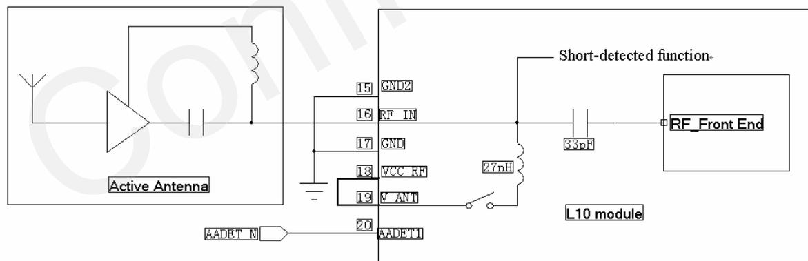
**Figure 14: Active antenna with VCC\_RF**
