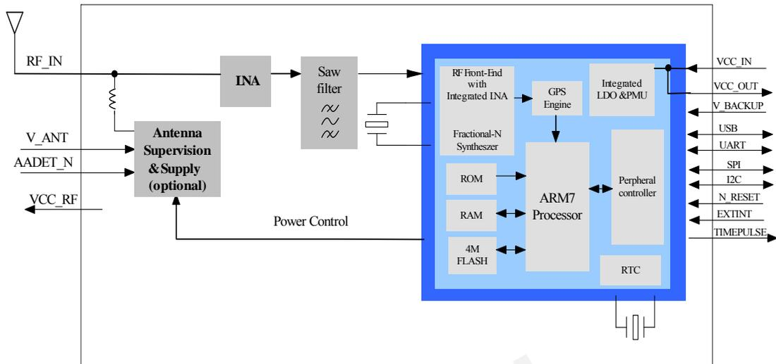
**Figure 1: Module functional diagram**
