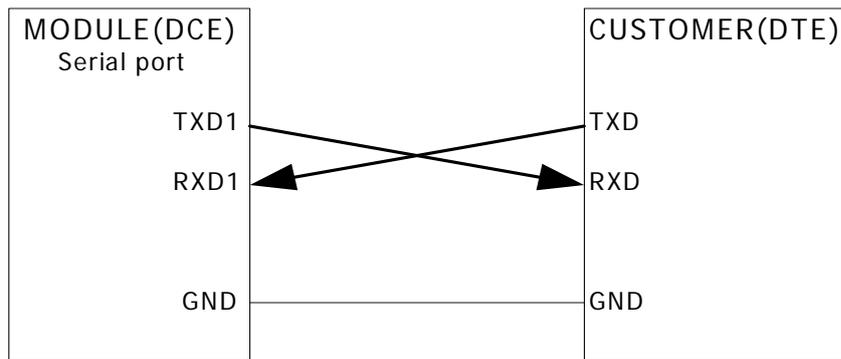
**Figure 8: Connection of serial interfaces**
