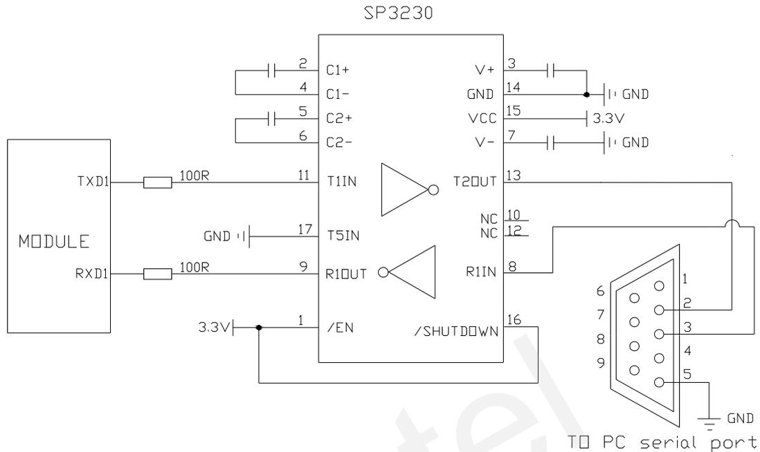
**Figure 9: RS-232 level shift circuit**
